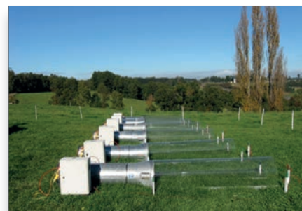
Figure 1 – Small wind tunnel technique used to evaluate ammonia losses following dairy slurry and urea application to permanent grasslands.
