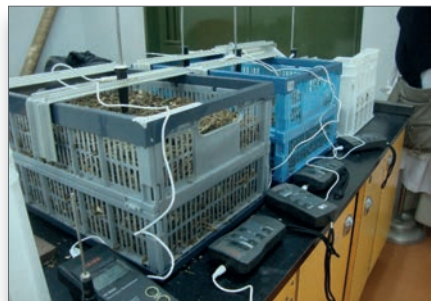
Figure 1 – Reactors with the compostable mixtures in the pilot plant
